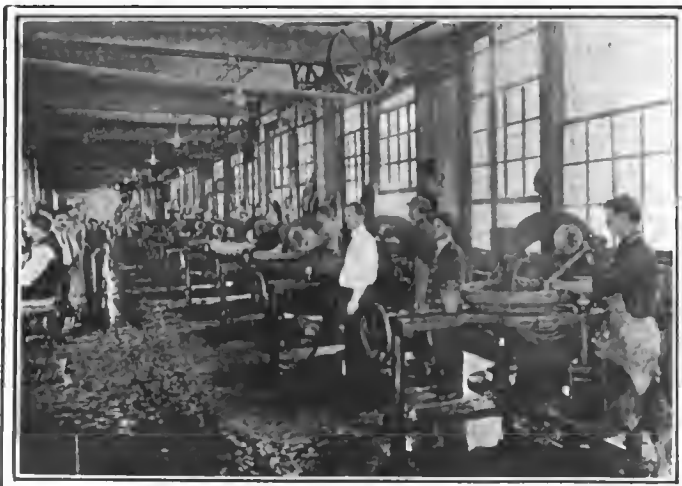
Wrapping room at the plant of the Goodyear Tire & Rubber Co., Akron, O. Here tires are wrapped prior to undergoing the second cure.
